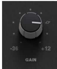
Turn the **GAIN** knob in the input section to control the level of the incoming audio signal. The post-gain signal level is shown above.
